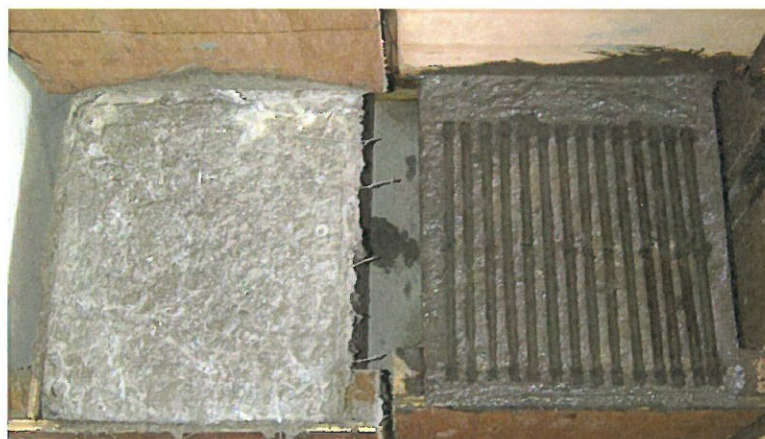
FIGURE 1: Difference of substrate surface conditions between as-placed and grooved with 6 mm of roughness amplitude
